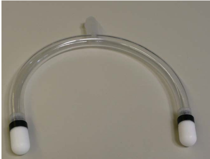
μ-sparger (PE; 18-45 μm)
